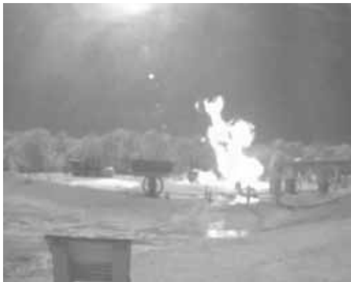
Light emission from the flame is viewed by the CCD array in the near IR. Flames appear in the picture as very bright objects against the background and this feature allows the FDS300 and FDS301 to discriminate against other radiant sources.
